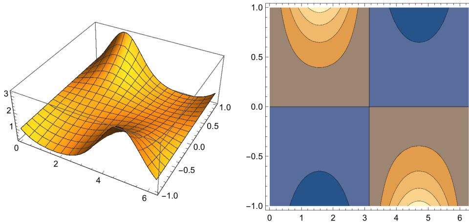
The working of the method of steepest descent (Sattelpunktsmethode) applied to the integrals above for large argument  $r$  can be understood in looking at the surfaces representing the modulus of the integrand.
