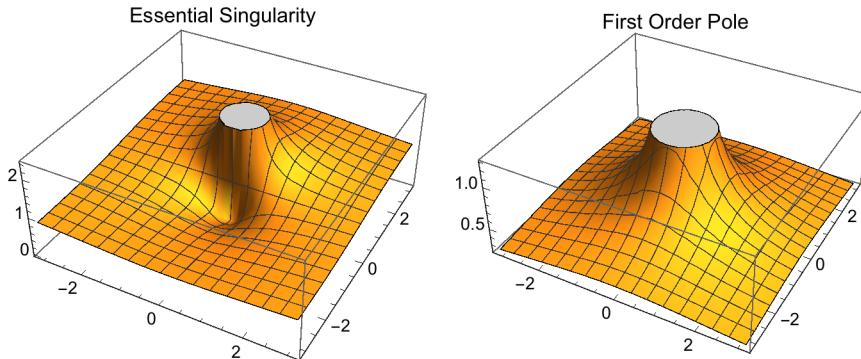
The preceding plots show the relief (= the surface of the absolute value of the function) of an essential singularity and of a pole.
