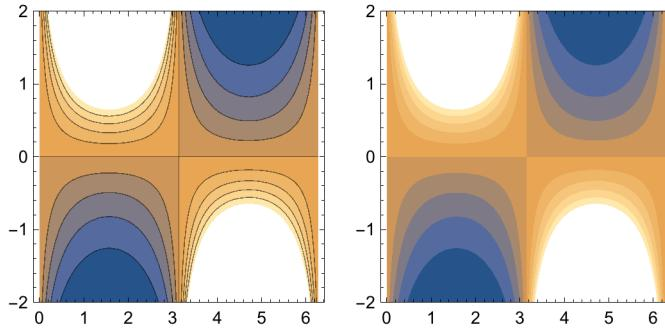
**Contours -> n** specifies to plot **n** contours, whose z values are spaced equally between the minimum and maximum z values. Default value **n** = 10.
