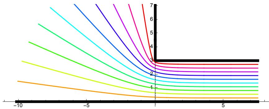
The figure above shows the equipotential lines for a configuration where a voltage is applied to the metallic electrodes shown in black.
