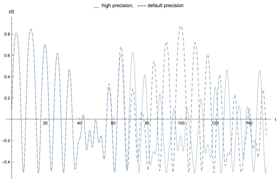
Diagrams in  $x,y$ -space are less suitable to show the difference between accurate and inaccurate solutions. From the outputs above it is seen that the options for higher precision entail about a factor 100 in CP time. The CP times, however, do not reflect the real running times, which last still longer. So other programming languages compare favourably for such tasks.
