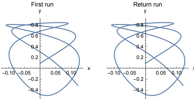
The solutions of this highly nonlinear system near the stability limit require appropriate options for runs over long time intervals; without these the solutions become inaccurate soon. But these options increase the CP time, the running time and data storage space very much. The accuracy is checked by running backwards from the end point to compare these end data with the initial data.
