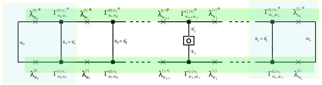
At the interior vertical lines, the spins  $s_i$  from the bra vector  $\langle \psi |$  and  $s_i$  from the ket vector  $|\psi\rangle$  meet. Since  $\langle s_i' | s_i \rangle = \delta_{s_i s_i'}$ , they have to be equal, except at the location j of the operator  $\hat{O}^{[j]}$ . Note that all lambda values are actually real, since they are singular values.
