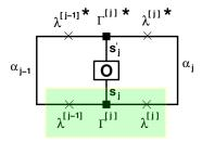
$$\langle \Psi | \hat{O}^{[j]} | \Psi \rangle = \sum_{s_j, s_j'} \langle s_j' | \lambda^{[j]} \Gamma^{*[j]s_j'} \lambda^{[j-1]} O_{s_j s_j'}^{[j]} \lambda^{[j-1]} \Gamma^{[j]s_j} \lambda^{[j]} | s_j \rangle \quad \text{with summations over the matrix indices alpha)}$$
