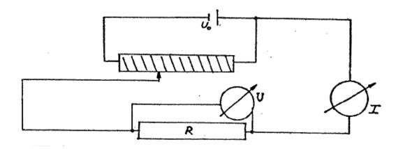
The data points (Voltage: V; Current I) follow **Ohm's law**, but are affected by an **experimental error**.
