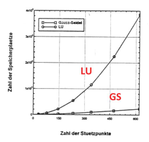
Efficiency of the G-S method compared to LU decomposition for a Laplace equation (sparse matrix).
