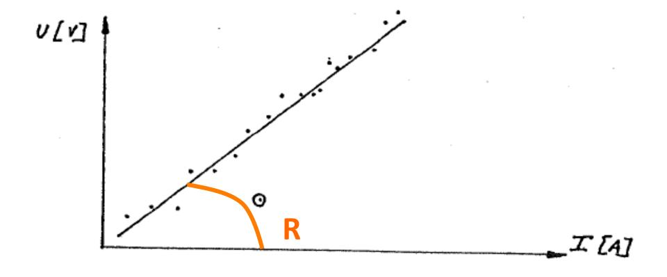
Due to experimental errors, the data do not lie *exactly* on top of a straight line (Ohm's law), but only *approximately*.
