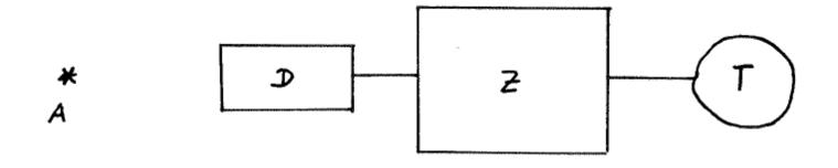
where A could be a radioactive substance, D a radiation detector, Z a digital counter and T a clock.
