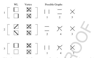
**Fig. 10.5.** Possible plaquette-graphs for vertex configurations. Graph one is a vertical breakup, graph two a horizontal one, graph four is diagonal. Plaquette-graph three is called frozen; it corresponds to the combined flip of all four arrows
