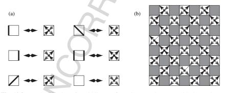
**Fig. 10.3.** (a) Identification of world-line configurations on plaquettes with the vertices of the six vertex model. (b) The world-line configuration of Fig. 10.1 in the language of the six vertex model
